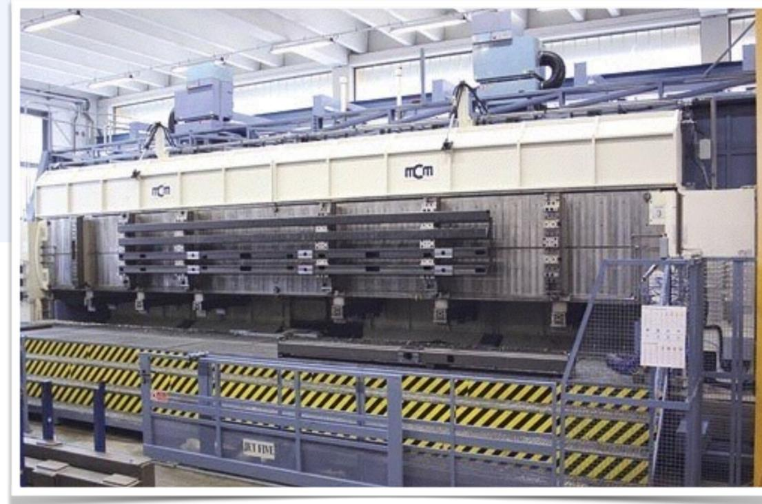
SMIMEC industrial plant is equipped with 20 CNC machining centers including 15 connected in FMS line that are able to carry out specific production programs even in the absence of operators.
